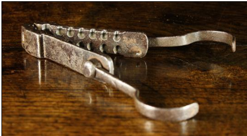
Figure 1. A gang mold capable of casting twelve lead shot. From A Woodrunner's Diary, 18TH CENTURY LIVING. HISTORY, HISTORICAL TREKKING, AND PERIOD WILDERNESS LIVING, http://woodrunnersdiary.blogspot.com/2016/04/more-on-small-shot-for-smoothbores.html
